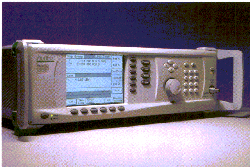
1. The MG8000A RF/microwave frequency synthesizer offers a broadband frequency range of 0.1 Hz to 40 GHz with low phase noise and various sweep modes.
